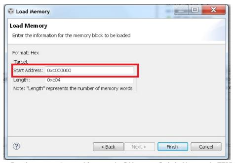
• Run the eepromwriter\_evmk2e.out on the C66x core to flash the binary to the EEPROM on the EVM.
