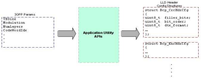
Figure 3. BCP header preparation
