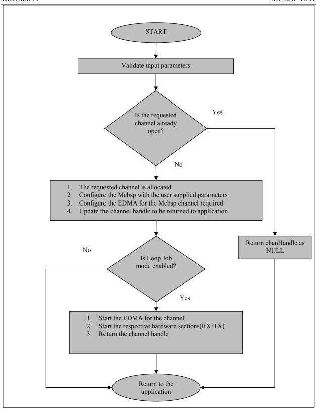
Figure 6: Create Channel Flow Diagram
