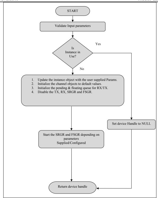
Figure 5: Driver Instance Binding
