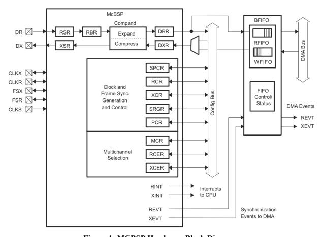
Figure 1: MCBSP Hardware Block Diagram
