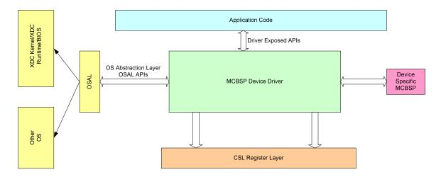
Figure 3: MCBSP LLD Driver Architecture
