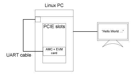
The test is verified on both TMS320C6670L and TMS320C6678L cards, with a 32-bit Linux PC running Ubuntu 10.04. Other 32-bit Linux OS are expected to work as well.
