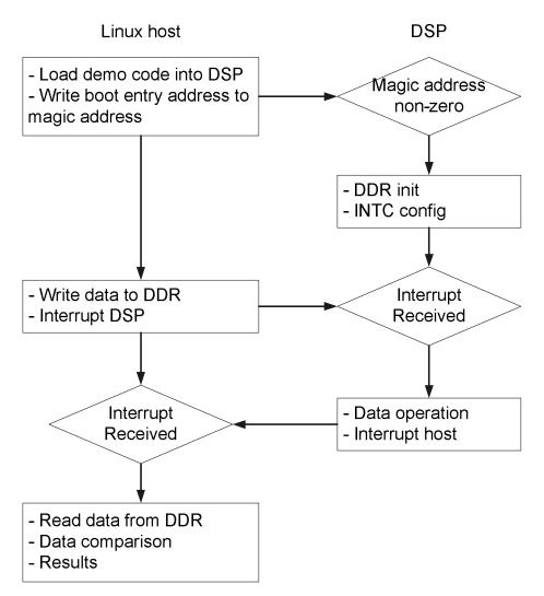
It is worth to mention that the EDMA over PCIE is implemented by poking the EDMA registers from the Linux PC via PCIE link. From DSP perspective, this is an outbound transfer as the local device (DSP) initiates the transactions to write to or read from the external device (PC). The HAL\_readDMA() function moves data from DSP to PC, this is outbound write from DSP's point of view. Similarly, HAL\_writeDMA() function is outbound read from DSP's point of view.
