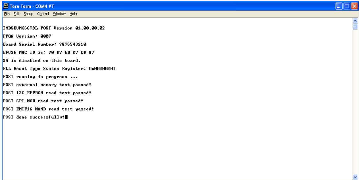
The screenshot shows a terminal window titled "Tera Term - COM4 VT". The window displays the POST (Power-On Self Test) results for a TMDSEUMC6678L board. The output text is as follows:
