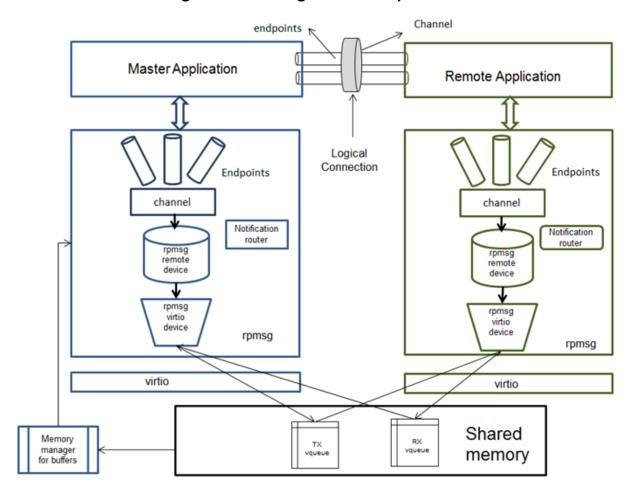
Figure 4-2. RPMsg Driver Components
